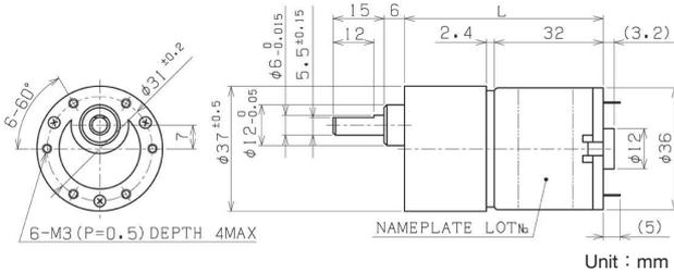
**RB-35GM-FMA11-24 DC24V** 起動電流 Starting current 940mA
